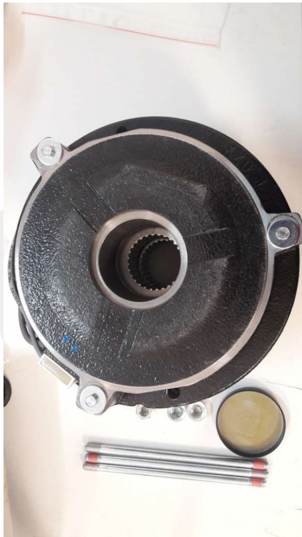
59601932 Brake assembly FCRD112 2X150 NM FMB130-LS-4C Schindler
